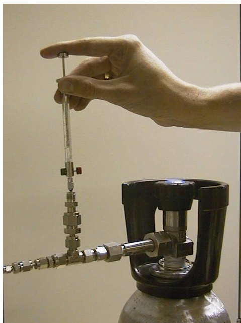
Figure D.1 — Example of introduction via syringe
